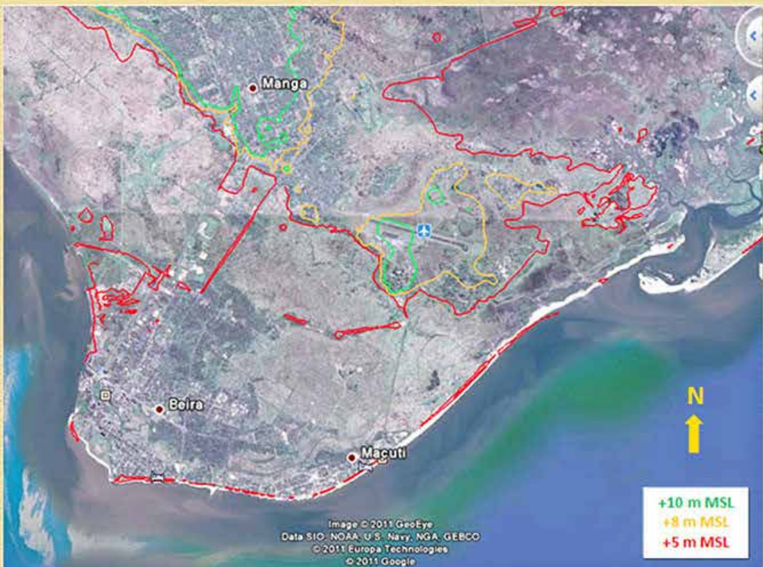
FIGURE 5. Satellite derived positions of the +5m, +8m and +10m (to MSL) contours at Beira city in Mozambique
